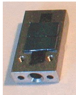
Figure 15: Sample Carrier Block loaded using silver DAG or double sided tape.
